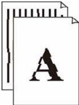
Lines Are Misaligned/Distorted
